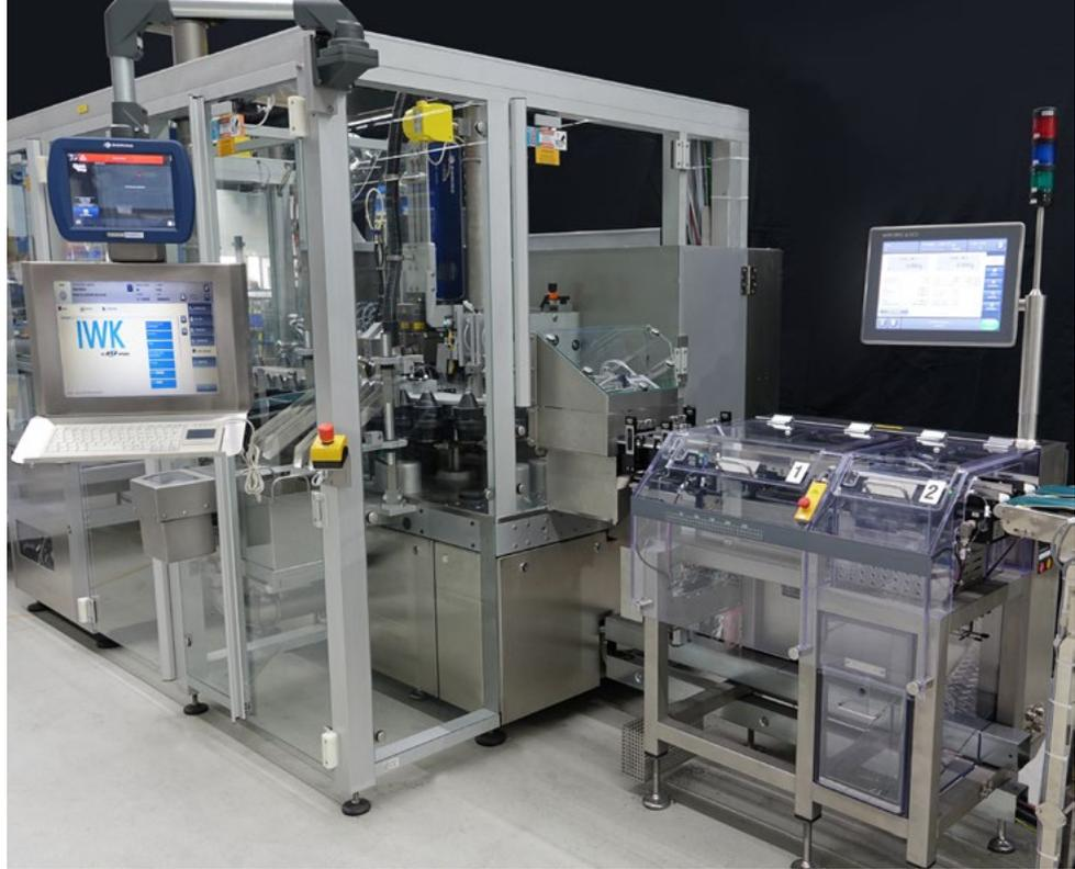
HC-A 2-lane Checkweigher solution downstream of the tube filler
