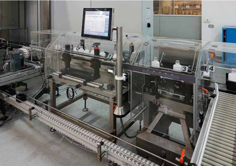
HC-A checkweigher with one-piece, RFID-equipped pucks for product transport.
