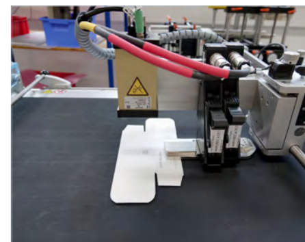
Print process of the non erected carton
