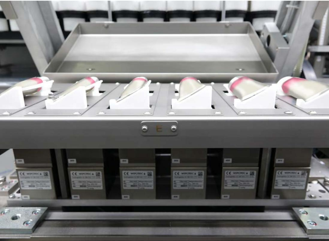
Pick & Place inline weighing as a cost-effective alternative to belt scales
